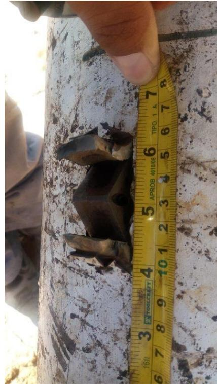
**CASING OPENING WITH BLADE**
