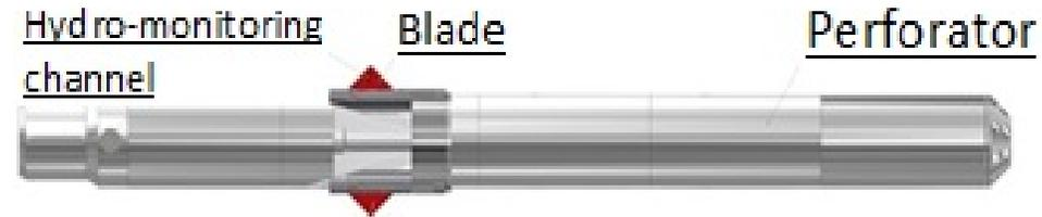
Piercing hydro-mechanical perforation is a part of second method formation perforation. The working method is the usage of hydraulic principles. The tool – is a hydro-mechanical device which working component consists of two sharp blades and four jet nozzles.
